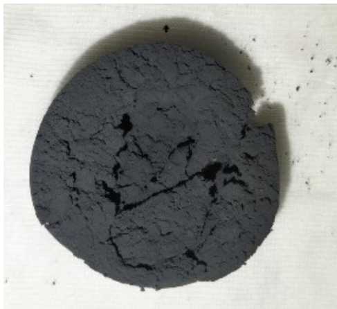
FIGURE 3. NMC 811 cathode active material product.
